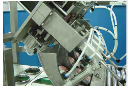
. Colocador de tapas no apilables . Non-stackable lids dispenser
